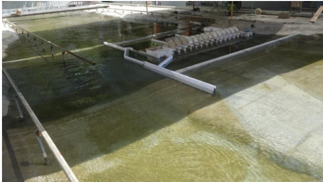
Flow pattern at a 20-year Flood ( Q=23174\text{m}^3/\text{s} )
