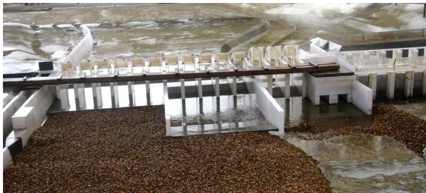
Scour Pit at Q = 39,040 \text{ m}^3/\text{s} (Full Opening of 2 Bottom Outlets + 14 Surface Bays)
